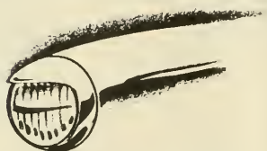
Round-type headlight with hooded bezel (rim of headlight)
